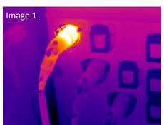
observable physical condition - temperature. Electrical connections become loose and the increase of the flow of electrons to that point manifests in a change in resistance with a resultant temperature increase that can be observed with an infrared imager. Likewise, an increase in friction on a bearing, belt, or conveyor can quickly be noted and scheduled for repair.
